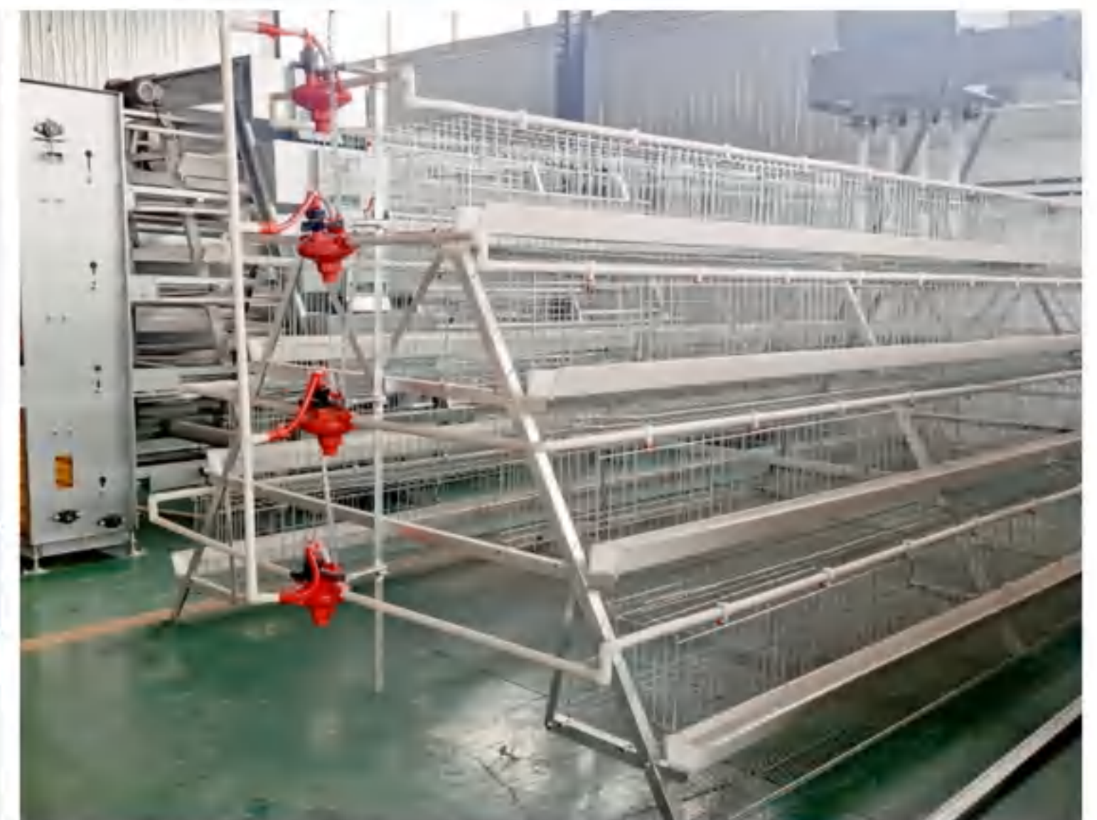
The specifications of layer cage ("HT" – Hightop® brand; "A" – A shape; "34" – 3 tiers 4 nests/doors; "L" – Large size)
